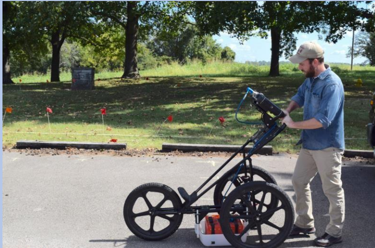
Using a ground penetrating radar (gpr) unit to search for the stockade Trenches at Garrison Hill
